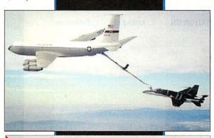
DUAL PERSONALITY Because Naval planes like this NASA F/A-18 use probe-and-drogue refueling, Air Force tankers like the KC-135 can refuel them only using an adapter on the boom.
