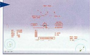
STEP 2: Close to 0.2nm and reduce closure to 30 knots.
